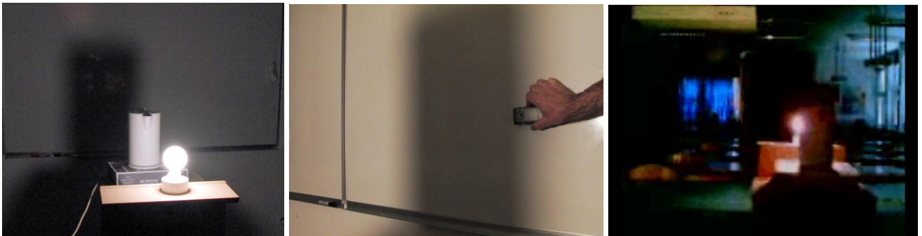
Figure 9: Examining a shadow by mobile phone camera: a) light source, object and the screen, b) moving mobile phone across the shadow region, c) view "seen" by the mobile phone camera as it passes across the penumbra .
